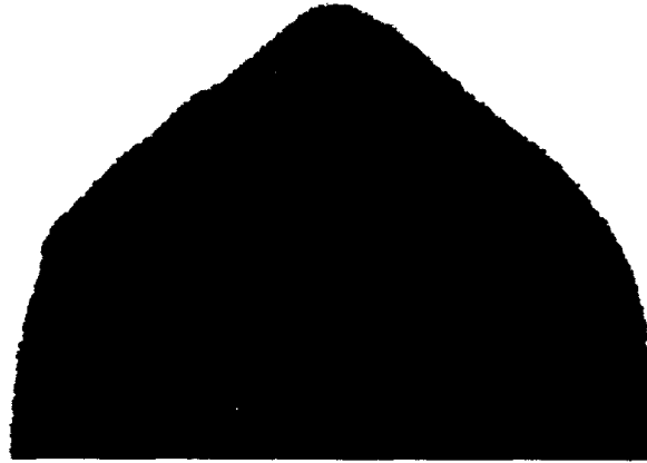
Fig. 4: Conical shape of the sample after the test with a pressure of 15 atm.
