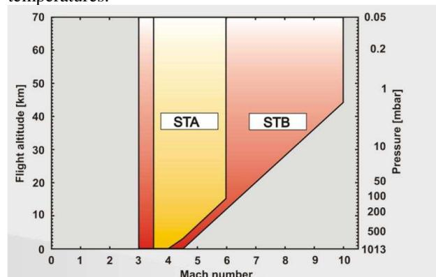
Figure 4: Capabilities of ISL shock tubes (credit ISL)
