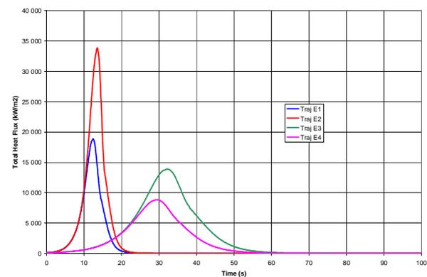
Figure 1: Total heat flux versus time for EVD mission [8].
