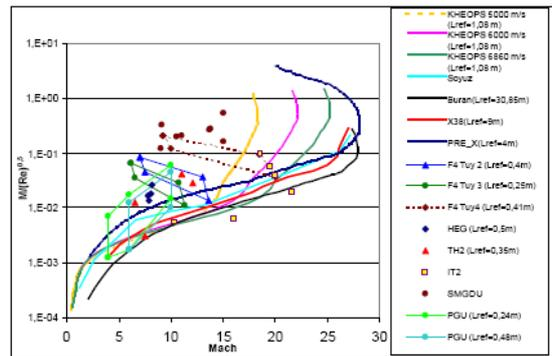
Figure 5: Capabilities of different facilities (F4, HEG, and TH2) for suborbital entries [2]
