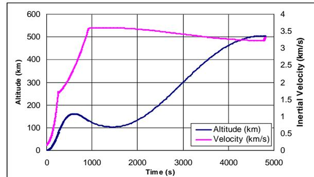
Figure 3: Typical Mars ascent trajectory [17]
