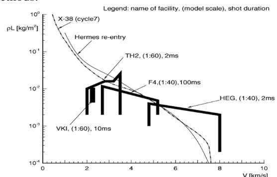
Figure 2: Performance envelopes of HEG, TH2, F4 and Longshot (VKI) for Earth suborbital re-entry according to Kordulla et al [9]
